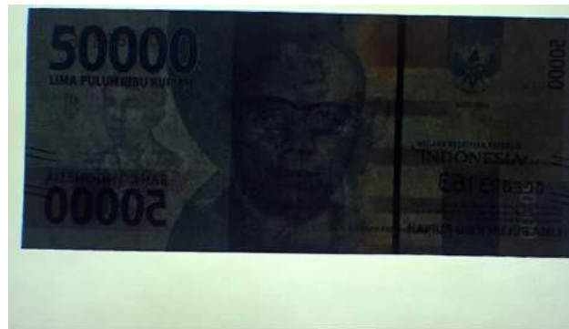
VSC3000 User, Default, VSC3000, Serial Number 11629 12/05/2012 16:55:50 Light=Transmitted, Longpass=VIS, Mag=1.89, White Balance=3720K 809RB Auto Exposure (Integration=3.2ms, Iris=50%), Brightness=50, Gamma=Off, Imaged width=159 mm
